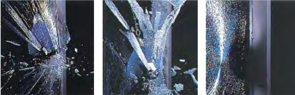
**ANNEALED GLASS** breaks easily, producing long, sharp splinters.
